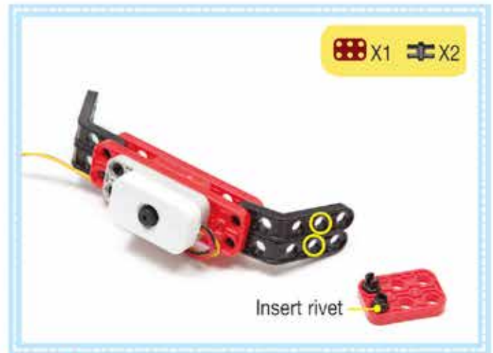
44 Assemble a 2X3 panel to the spotted points of the V-bracket.
