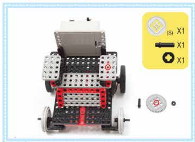
35 Insert a rod rivet into the spotted point of the 3X5 panel and fix a gear(s) to the rod rivet. Fasten it with a bushing.
