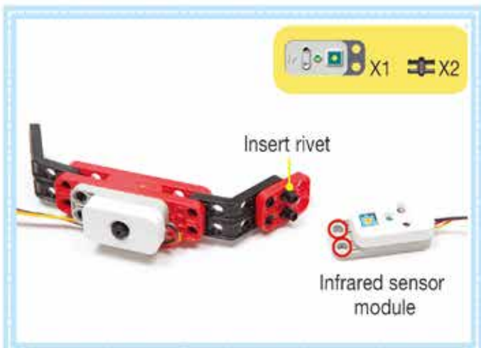
45 Assemble an Infrared sensor to the 2X3 panel.
