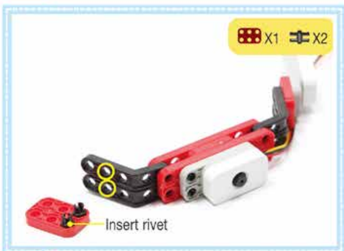
47 Assemble a 2X3 panel to step 46 .
