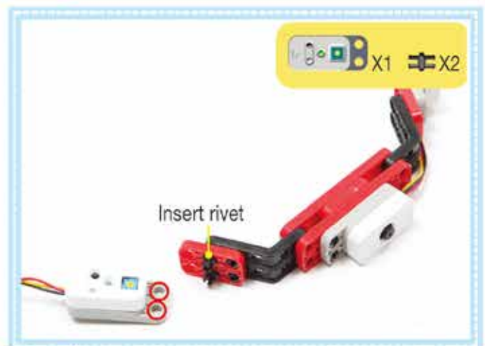
48 Assemble an infrared sensor to 2X3 panel.
